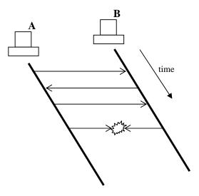
Figure 1: Collision in the Basic Aloha Protocol
