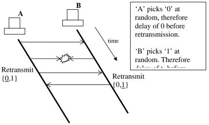
Figure 2: Retransmission in the Basic Aloha Protocol
