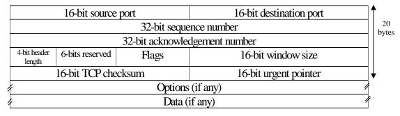
Figure 4: TCP Header [8]
